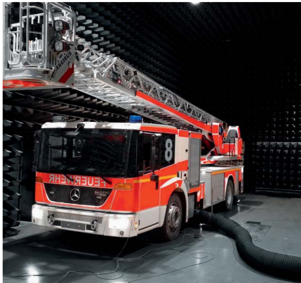
/ Ladder in EMC test
